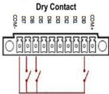
**Note:** If you are using wet contacts, you must connect COM to power.
