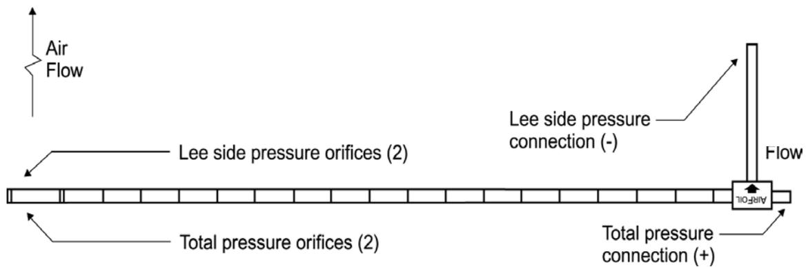
FIGURE 6.2 AIRFOIL PROBE
