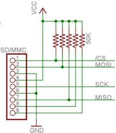
Remark: this schematic includes pull-up's to 3.3V, which can be left off.
