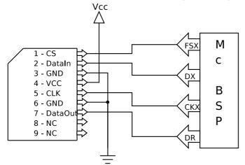
The frame sync from the McBSP port is used to select the card whenever a databyte has to be transferred, it is connected to the chip select of the SD card. The DX and DR pins are connected to the SDcard's DataIn and DataOut lines respectively. Finally the McBSP will have to generate a clock for the SDcard so that it can perform operations, this is accomplished by connecting the clock transmit line of the McBSP port to the CLK pin of the SDCard.
