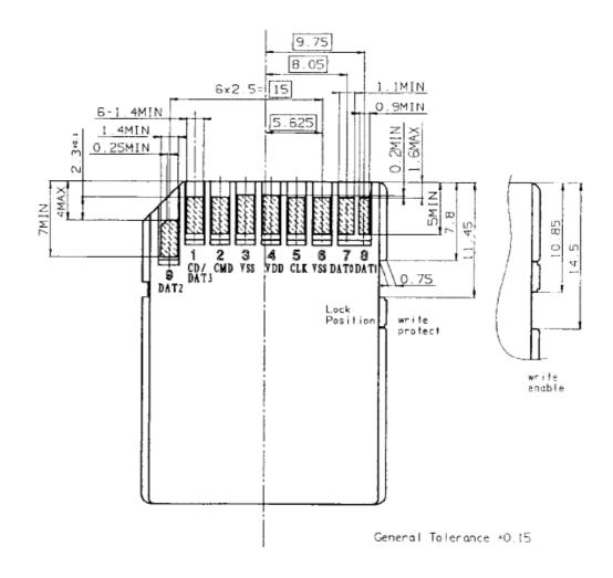
Connect the following lines on the SD-card:
