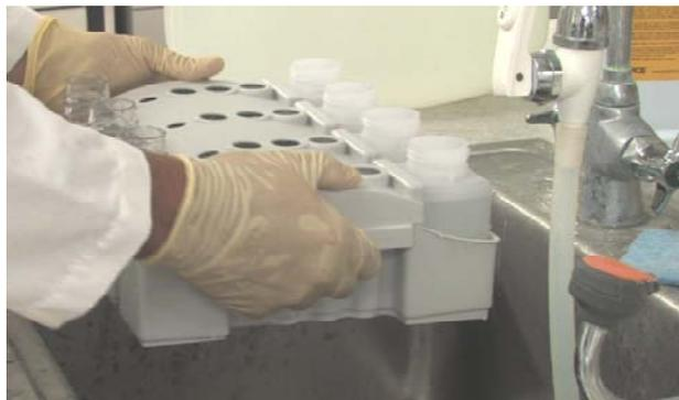
5. Remove the Waste Basin and discard the waste appropriately, if the auto-drain feature is not used. Transport the waste reagents carefully to sink to avoid any spillage. Rinse the Waste Basin with water prior to use.
