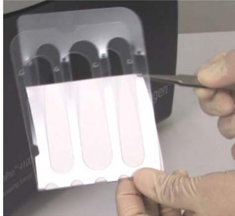
6. Holding the sides of the Blot Holder together, slide the Blot Holder containing the membrane into the blot chamber of the card. Transfer membrane insertion is easier if the card is already inserted into the instrument.
