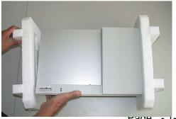
When setting up the reader, take care not to grasp the device at the top near the (closed) scanner cover but only at the back housing cover and below at the base plate.
