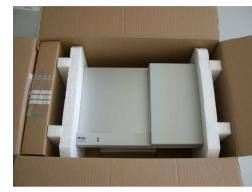
♦ Grasp the reader by the filling materials mounted on the left and right sides of the device and lift it carefully, straight upwards out of the cardboard box without tilting it. The device weighs about 6 kg.
