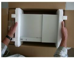
♦ Set the reader down on the intended work surface and remove the two pieces of filling material on the sides.
