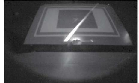
6. Turn the adjusting knob **3** clockwise until the reflection line is horizontal.
