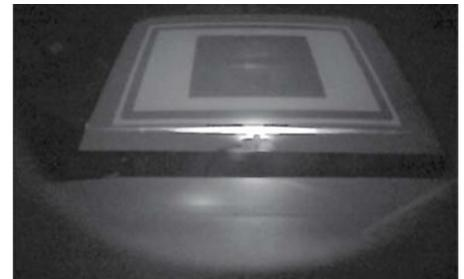
7. Turn the adjusting knob **1** clockwise so the reflection line moves near the vertical center.
