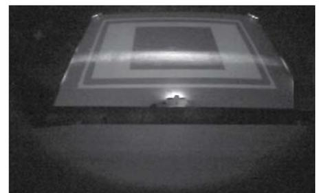
9. Turn the adjusting knob **1** counterclockwise until two adjusting bars each appear at the bottom right and left of the screen. You are looking for two white dots on either side.
