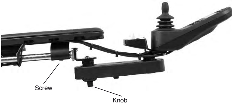
Control panel with parallel panel holder.
