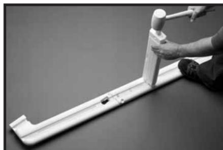
**#1:** Lay outside rail assembly on flat surface so that the notch in the hooked end is facing up. Insert tread into the opening second from the top and tap down. **NOTE:** The notch located on the top surface of tread must face inward towards the "hook" side of rail.
