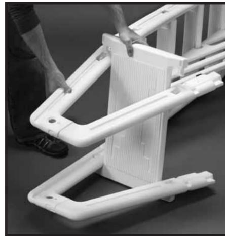
**#10:** Slide one tabbed end of the platform under the return rails closest to the floor. Flexing the top rail assembly downward slightly, slide the platform toward the top of the ladder until platform tabs fit into the locking holes in the rails.
