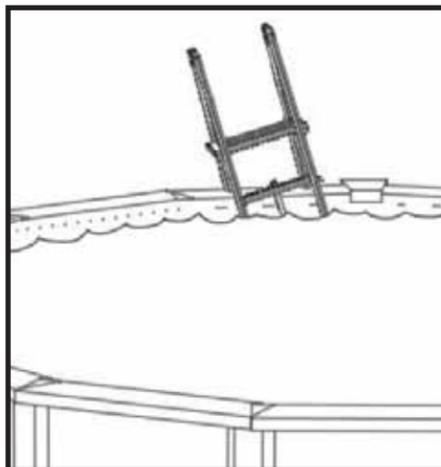
**#2:** Position ladder where it will attach to deck. Make sure bottom tread of ladder sits firmly on pool bottom. Slide the adjustable rails so mounting blocks sit flat against the deck.
