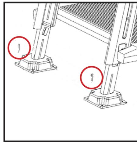
**#3:** With the cordless drill secure each mounting block to the deck using four #10 x 1-1/4" self-tapping screws.
