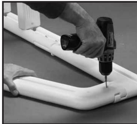
**#9:** Attach rails using two #10 x 1-1/4" self-tapping screws (one in the designated mark on the inside rail and one on the outside rail). Flip ladder assembly over and repeat with remaining return rail.
