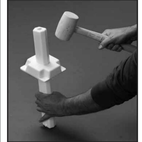
**#3:** Turn mounting block assembly over and tap the mounting block down the adjustable brace until it is seated snugly at the base of the brace. Repeat for other mounting block assembly.
