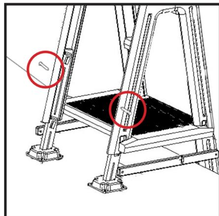
**#4:** Making sure the platform is level, secure the return rails to the mounting block tubes by inserting four #10 x 1-1/4" self-tapping screws at the marked locations (two screws per rail).
