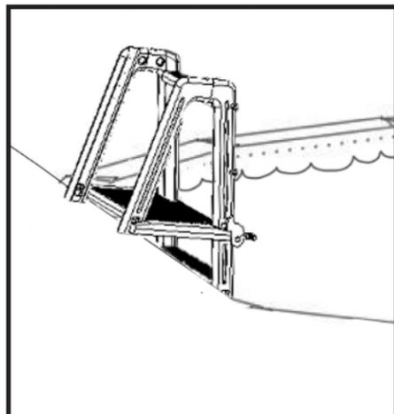
**#1:** Place your ladder inside the swimming pool. Using a garden hose fill both rails through the openings located on the top of hand rails. Tilt the ladder from side to side to get all the air out of treads. **NOTE:** Ladder treads must fill with water to prevent floating. Cap when filled using white plugs provided.
