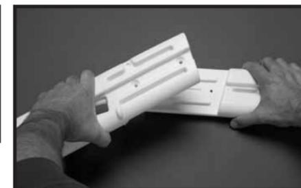
**#1:** Place Lower Side Rail on a flat surface with notched end facing up. Place Upper Side Rail notched side down so it overlaps the Lower Side Rail and both pieces fit together smoothly.
