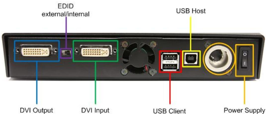
Connect the workstation PC (source) to the 'DVI in' connector. The Signal is loop trough to the second DVI connector which is marked with 'DVI Out'. With the switch between the connectors the EDID information that is been transmitted to the attached source can be selected: Either the internal EDID, stored on the eS100 or the EDID information of the attached Monitor on the 'DVI Out' connector.
