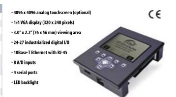
The OP7200 eDisplay is an ideal data acquisition operator interface SBC that offers rugged I/O, built-in Ethernet connectivity, and optional A/D and touchscreen capabilities. It is ideal for data acquisition, display, and control. Two eDisplay models incorporate 24-27 digital I/O plus an I/O expansion port and 4 serial ports. When frontpanel mounted, the unit meets NEMA 4 water-resistance standards, making it suitable for use in harsh environments.
