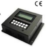
The Intellicom is a 12-key graphic display with optional Ethernet for network connectivity and a VFD option for applications requiring high visibility. To accommodate users' installation preferences, the versatile Intellicom can be either wall or panel mounted. The OP6700 offers direct connection to 10Base-T Ethernet and communicates with serial devices via RS-232 and/or RS-485, providing multiple solutions for communications applications. Eight general-purpose I/O provide control functionality.
