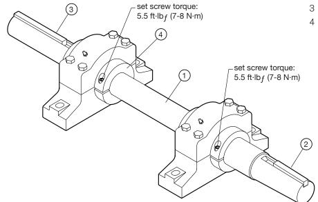
**Installation:** Installation should only be performed by a qualified technician. Lockout and disable any system drivers. Coat the shaft(s) with a lubricant or anti-seize compound. Follow the instructions supplied with your replacement kit or the tower User Manual. Contact your Marley sales representative should you need more information for your application.
