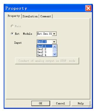
The SMS input used as same as other modules of ELC series. It is a digital input.
