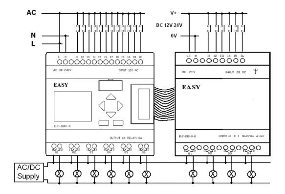
Notes: 1. ELC-SMS-D-R can be connected to any voltage class ELC-18 series CPU module.
