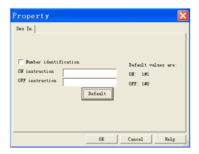
The SMS message inputs can be controlled by an SMS i.e. they can be switched ON and OFF. Each SMS message input can be activated individually. The message text can be chosen with Arabic numerals or English words. However the device only reacts to the exact expression i.e. the message must correspond exactly with the inputted expressions.
