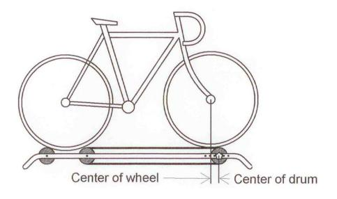
Your roller comes completely assembled. Unfold the unit and set the belt into the grooves on the front drum and the middle drums so that the middle drum drives the front drum smoothly.
