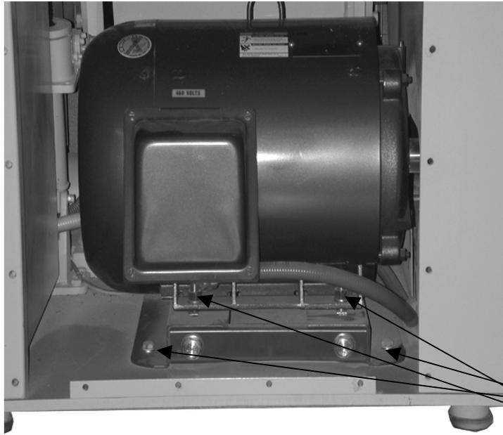
Loosen these 4 nuts on the bolts holding the unit on the base. Slide the motor either backwards or forwards to achieve the proper belt tension and retighten the nuts.
