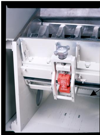
Optional Airveyor should be inserted into these clips located on either side of the unit.
