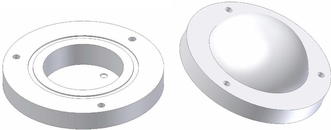
**Figure 3.15** Isometric view of the inside and outside of the bottom cap.
