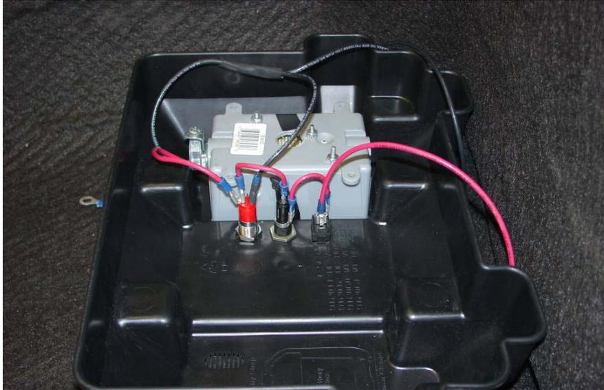
**Figure 3.20** Surface component junction box mounted to the underside of battery box lid.
