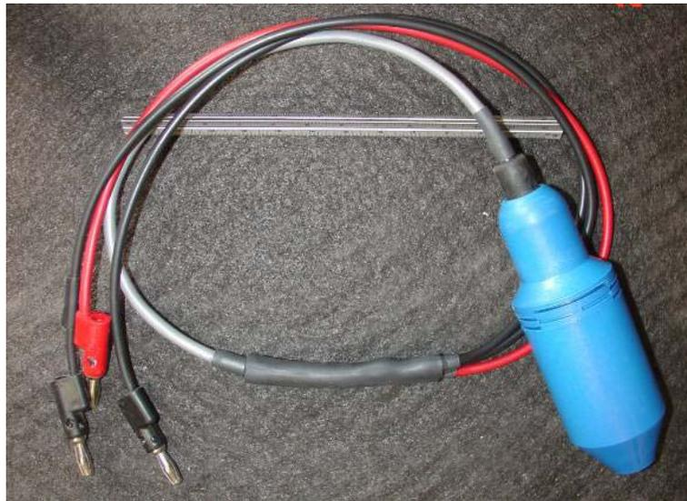
**Figure 3.27** Assembled geophone ready for field use.
