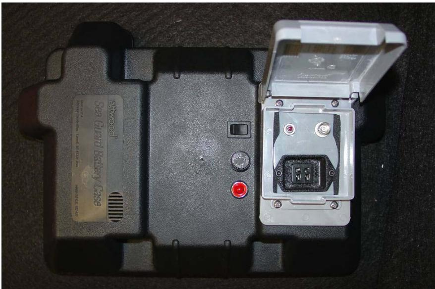
**Figure 3.21** Finished battery box.
