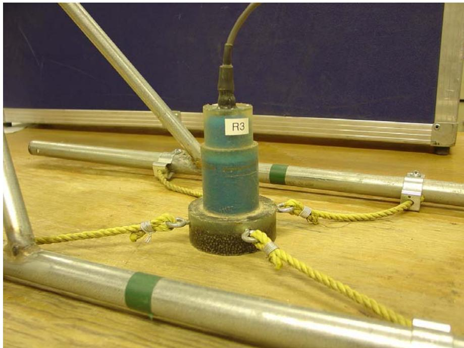
**Figure 3.29** Finished de-molded potted geophone.
