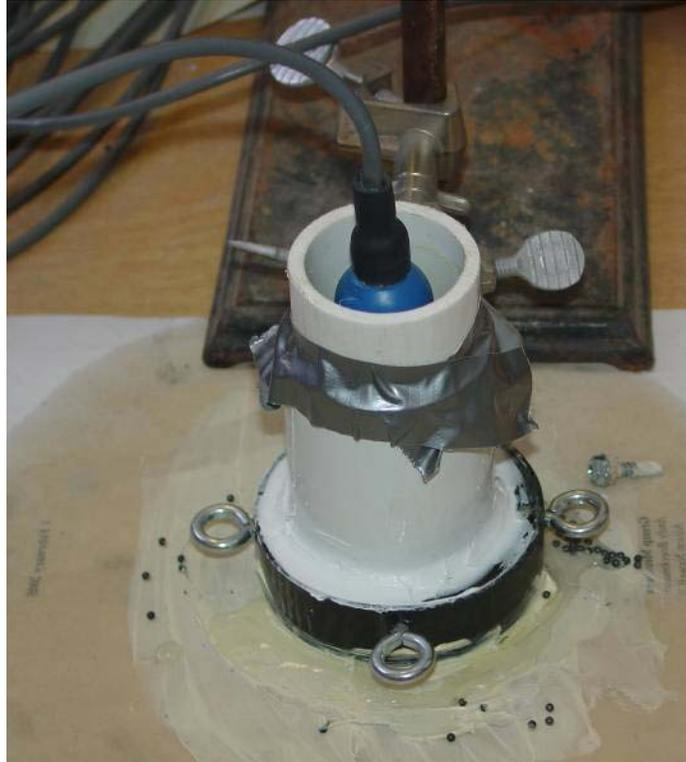
**Figure 3.28** Intermediate step in geophone potting.
