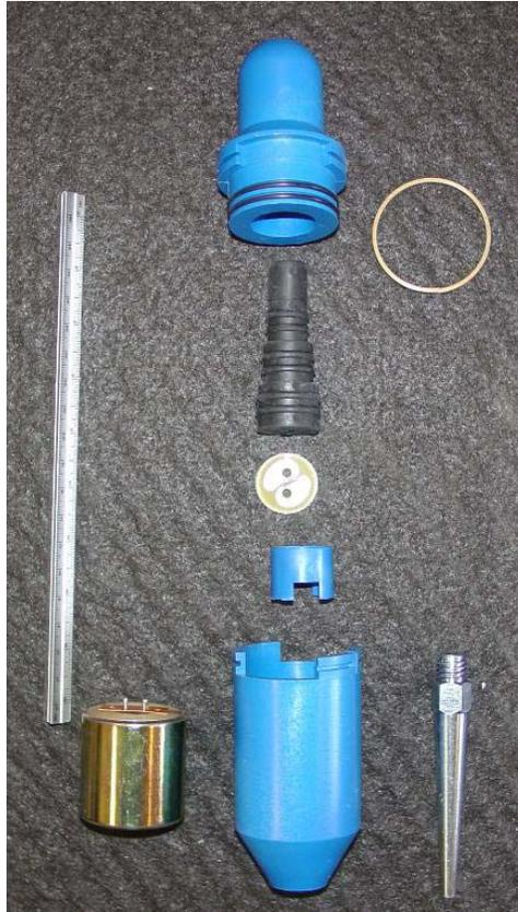
**Figure 3.26** Geospace LP 4.5 Hz geophone and marsh case assembly.
