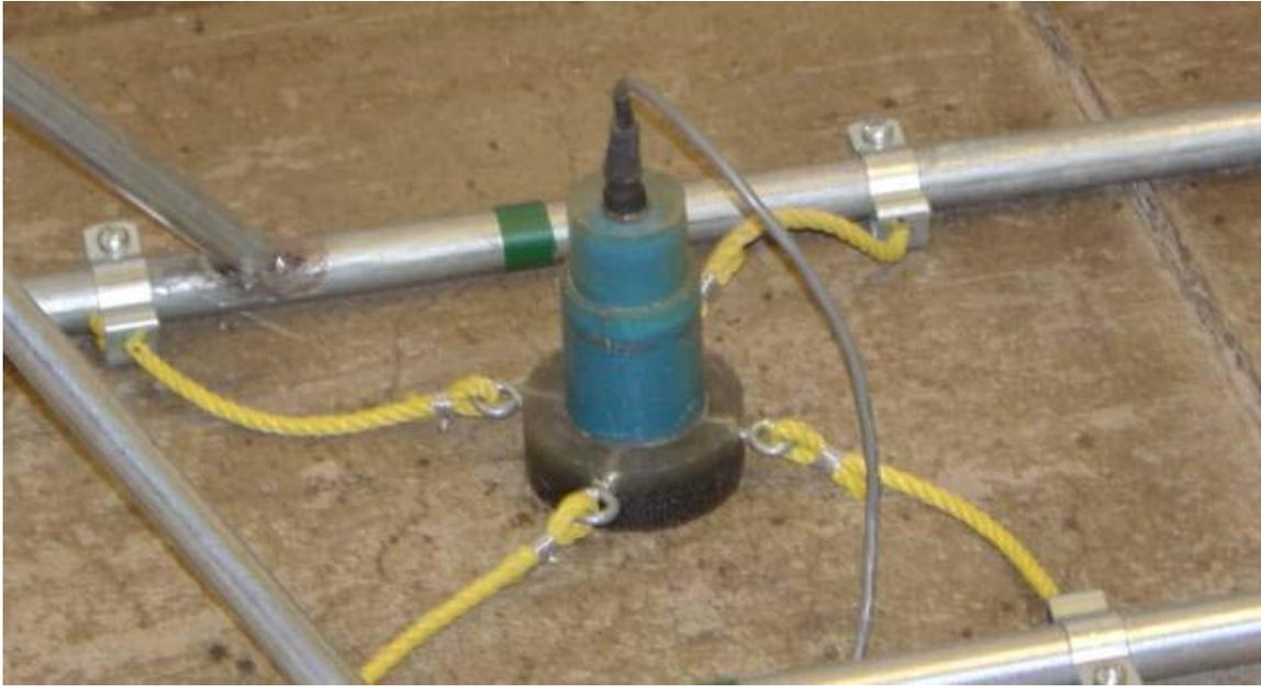
**Figure 3.31 Geophone mounted in frame with hardware.**
