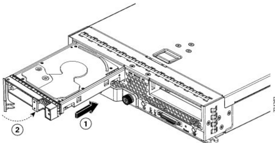
**Step 2** Gently slide the hard drive into the opening in the blade server until it seats into place.
