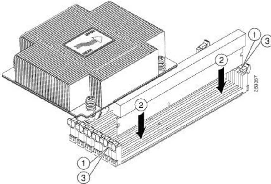
**Step 2** Press the DIMM into its slot evenly on both ends until it clicks into place. DIMMs are keyed, if a gentle force is not sufficient, make sure the notch on the DIMM is correctly aligned.
