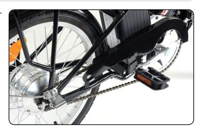
To tighten the chain, undo the axle nuts a little so that the axle is free to move, and then do the
