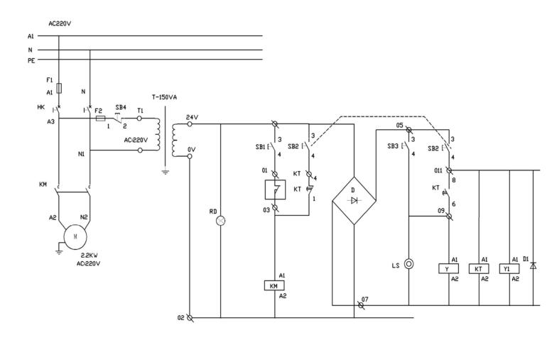
SB1~3--button KM-contavtor B16 AC:24V T-transformers AC:220V/24V-26V
