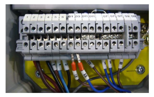
3.3.6 Connect the power supply plug in accordance with the electrical schematic diagram, then connect the compress air (the range of air pressure is between 1.0 and 1.5 kg/cm2) to air inlet of pump station oil-water separator, and then connect security lock pipe to the air outlet of pneumatic solenoid valve of pumping station.
