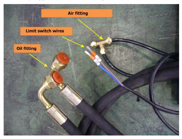
3.3.3 Indentify the pipe and wires, as shown in the figure below.
