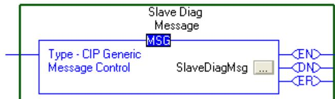
Figure 20 : “MSG” Instruction with SlaveDiagMsg
