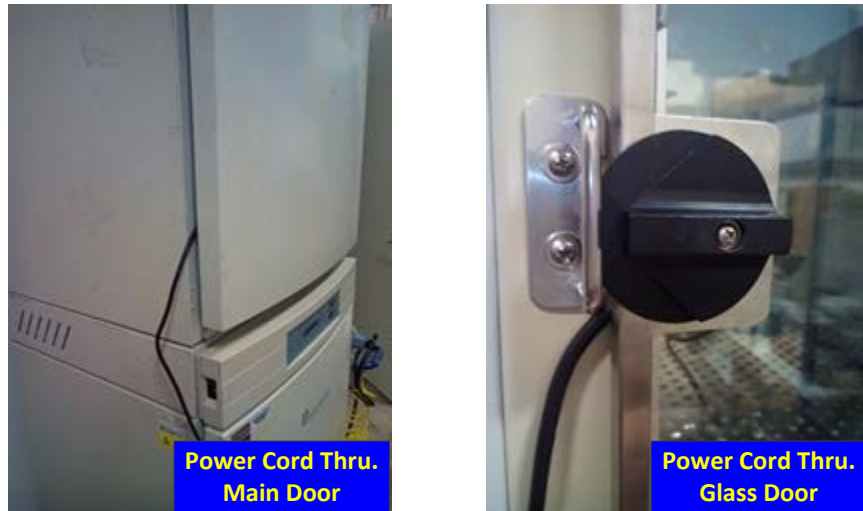
Figure 10. Pump’s Power Cord Through Incubator’s double doors
