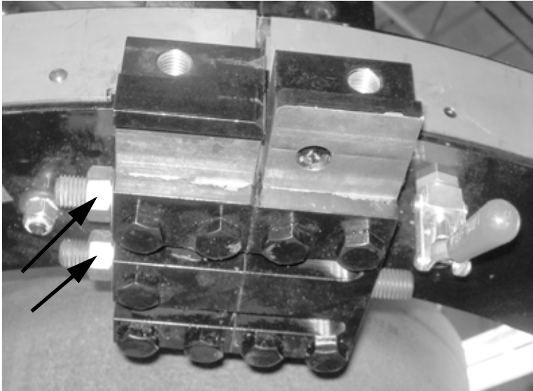
Figure 7-3. The photo shows the swing latches on the stationary ring side of the frame. Loosen the nuts and lift the latches out of their channels.
