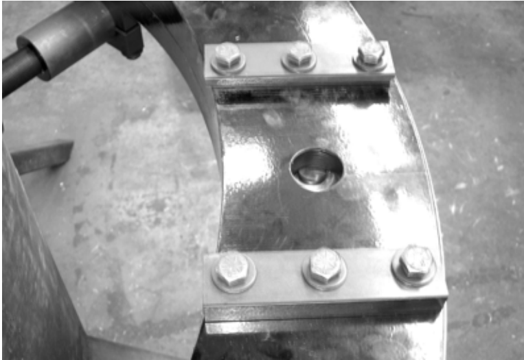
Figure 5-14. Install the slide mounting blocks on the rotating ring. Leave the mounting bolts loose.
