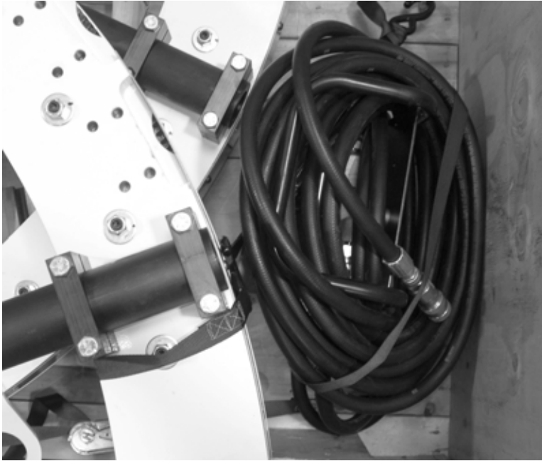
Figure 4-7. Put the flow control assembly along the side of the case.
