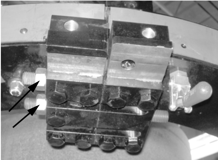
Figure 5-4. The photo shows the swing latches on the stationary ring side of the frame. Loosen the nuts and lift the latches out of their channels.
