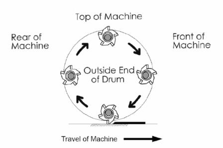
Correct rotation of the Milling Cutters is critical to successful resurfacing and to insure maximum wear life. Drum and cutter assembly should be mounted so that cutters are rotating towards the front of the machine as indicated above.
