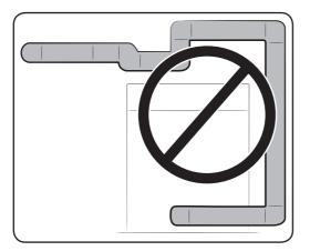
**3.** Using unnecessarily long ducts that have many elbows.
