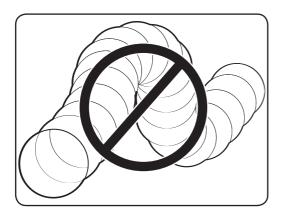
**2.** Using a plastic, thin foil, or non-metal flexible duct.
