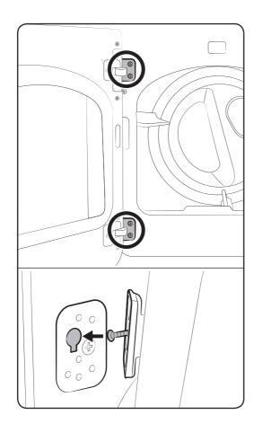
**16.** Install the door on the frame-front and then fasten the 4 screws that you removed in step 2.
