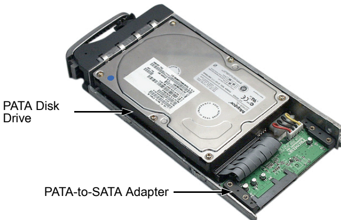
Figure 5. PATA Disk Drives require a PATA-to-SATA adapter
