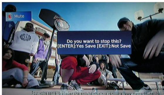
A dialogue box will be displayed on screen asking you to confirm. Press “OK” to stop the TIMESHIFT, To save the space of the USB hard drive, the recorded program is not stored under time shift mode.
