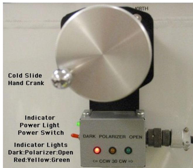
Fig. 13 Cold Dark Slide hand crank and indicator
