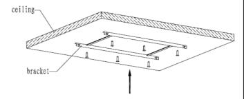
Position the heater onto the bracket
