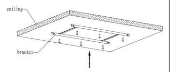
Position the heater onto the bracket
