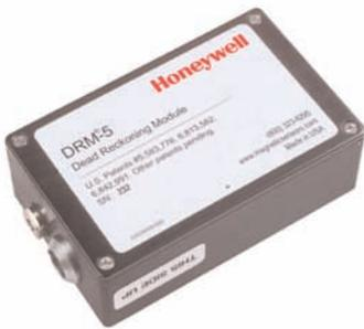
A development kit is available and includes: a 16-channel GPS receiver, antenna, all dead reckoning functions and sensors, waterproof housing attached to a web belt, long-life Li-Ion rechargeable battery, Windows® based test and demonstration software, and user manual. This is an ITAR restricted product and requires an export license to ship outside the United States.
