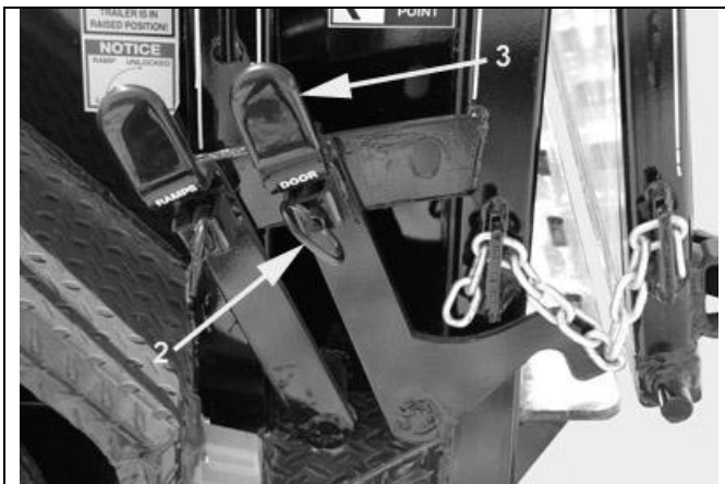
Unlock Spreader Gate - Figure 5-5
