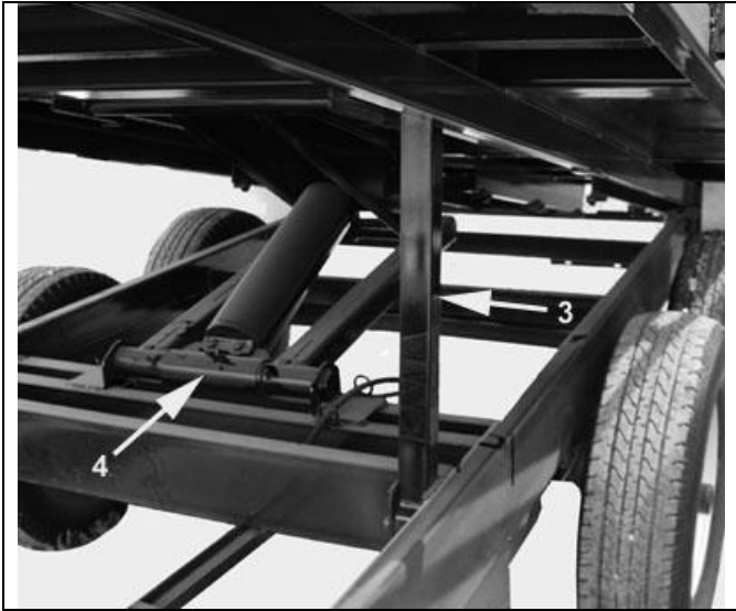
Support Body and Lubricate Cylinder Ends - Figure 11-3
