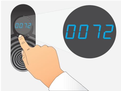
**STEP 3:** Compose the desired locker number by pressing the 'up' key to increase or the 'down' key to decrease the currently flashing digit. Use the 'enter' key to move to another digit. When you get to the last digit, pressing the 'enter' key will return the focus to the first digit.
