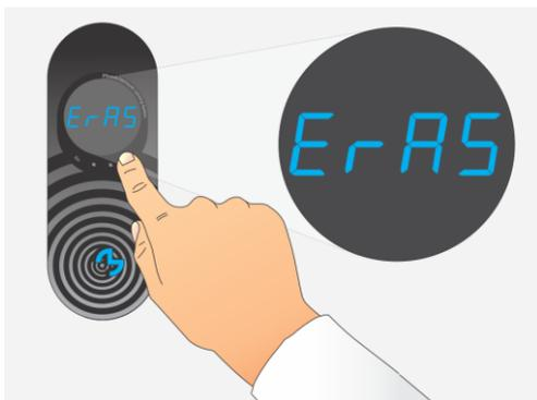
**STEP 3:** Press and hold the “Enter” key until “ErAS” is displayed and short “beep” acoustic signal is activated.
