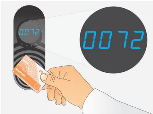
**STEP 4:** When desired locker number to be opened is displayed, present the Master Card again to the antenna field to confirm unlocking.
