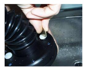
7. Turn up the electrode and check once more the appropriate volume of the water in the bolus and that it is de-aerated. .
