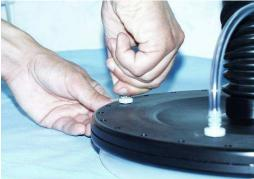
Before the opening of the filling up hole, put a tray or absorbing textile below the electrode to avoid the water to overflow.
