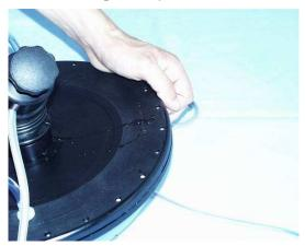
6. Put the electrode in the horizontal position. Ask for help to hold the electrode. Push the bolus up with one of the tip of your fingers til you reach the electrode metallic plate. The access water is taken off from the bolus with this procedure.
