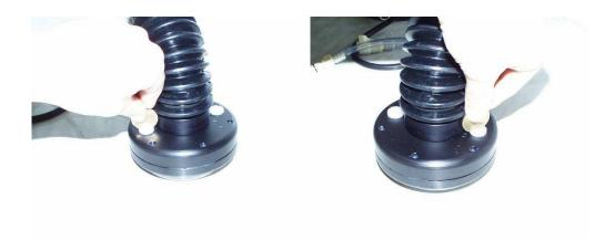
Before the opening of the filling up hole, put a tray or absorbing textile below the electrode to avoid the water to overflow.
