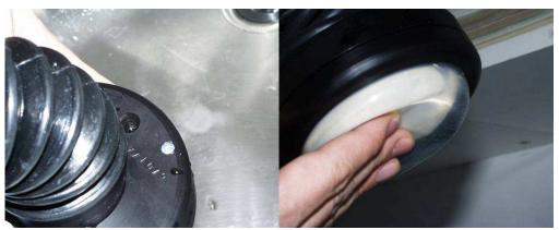
Take care that during this process air must not enter into the bolus. Take care that you can continuously see the water in the filling hole. Just in this position screw tightly in the packing nut.
