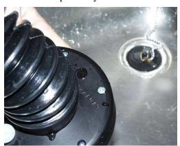
6. Put the electrode in the horizontal position. Ask for help to hold the electrode. Push the bolus up with one of the tip of your fingers till you reach the electrode metallic plate. The access water is taken off from the bolus with this procedure.
