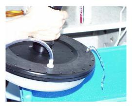
Take care that during this process air must not enter into the bolus. Take care that you can continuously see the water in the filling hole. Just in this position screw tightly in the packing nut.
