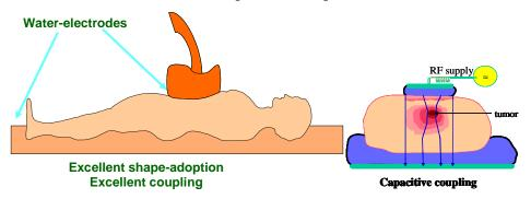
The patient's individual shape is corrected for planparalel electric condenser with transmitter fluid.
