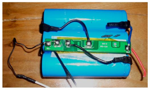
Figure 8: This balancing circuit keeps the individual cell voltages the same and is the reason external balancing mode is selected when charging these batteries. Some lithium ion batteries come with a built in thermistor to sense battery temperature. A thermistor is a type of resistor whose resistance varies detectably with temperature. If battery temperature is not an issue the white wire can be disregarded/cut.
