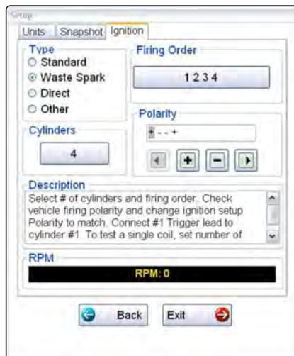
Figure 8-30 Sample Setup Ignition dialog box
