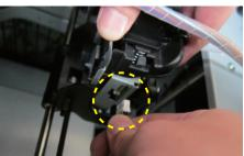
4 Unplug the heating bus at the side of the extruder module
