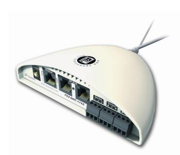
The Networked Room Controller (simplified in this paper as "NRC") acts as a central hub within a room for control of projectors, monitors and other equipment, offering webenabled control of any display device. Measuring only 1.44" H x 5.44" W x 4.5" D, the NRC can be mounted completely out of the way in a classroom without taking up any valuable rack space. The NRC is the only AV controller that is compatible with the wildly successful annotation and teaching app and software Doceri.
