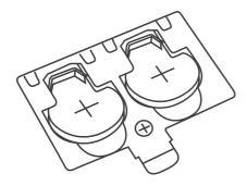
Install Both CR2302 Batteries Positive Side Up
