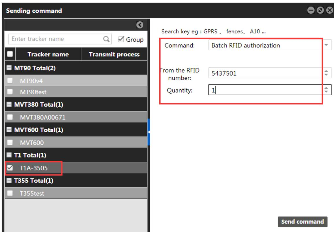
The screenshot shows the 'Sending command' window. On the left, a table lists trackers with columns for 'Tracker name' and 'Transmit process'. The 'T1A-3505' tracker is selected. On the right, the 'Command' is set to 'Batch RFID authorization', the 'From the RFID number' is '5437501', and the 'Quantity' is '1'. A 'Send command' button is located at the bottom right.
