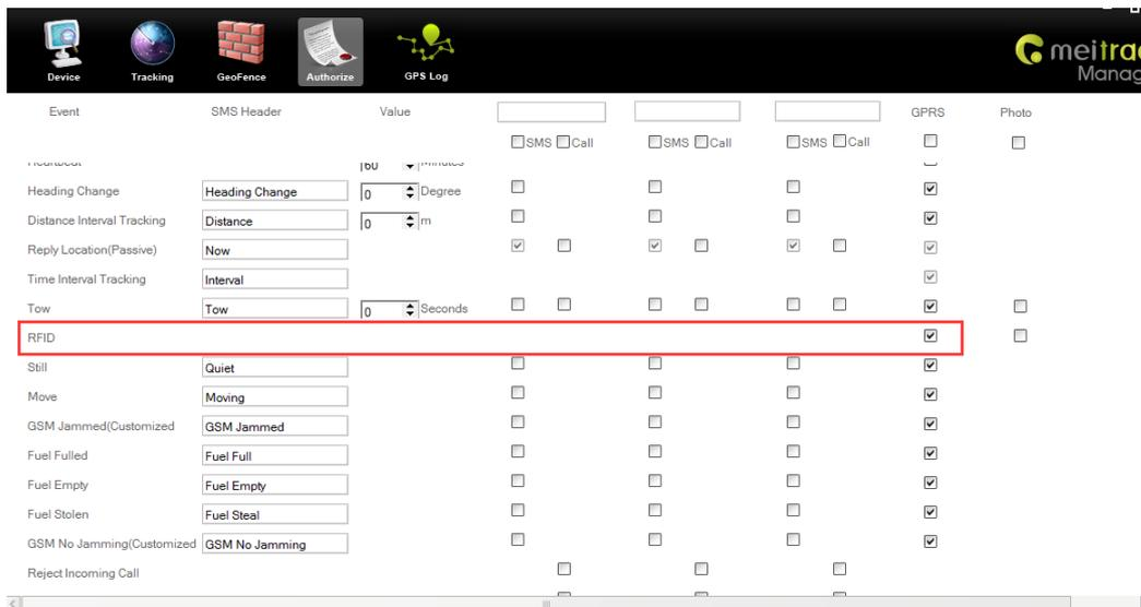
Note: If this RFID option is deselected, the MS03 platform cannot collect statistics on RFID event reports after you swipe a RFID card. The RFID event is enabled by default.
