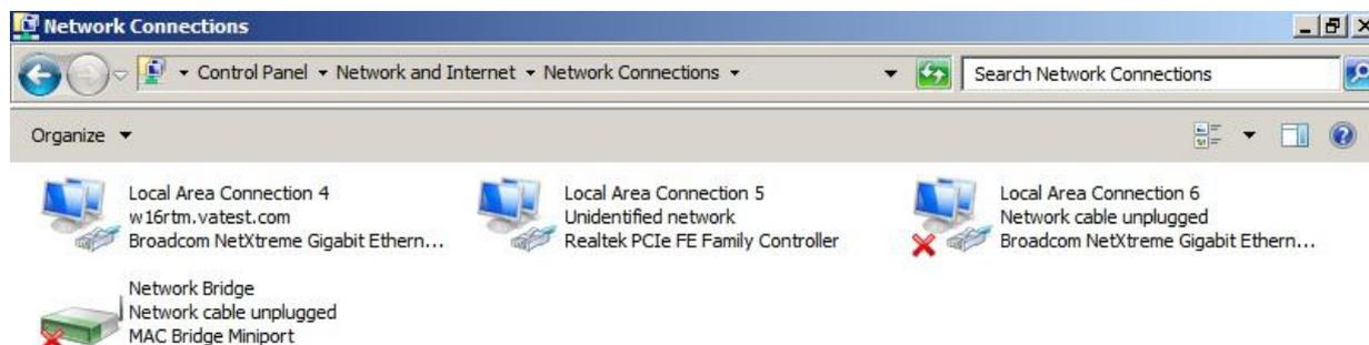
Image 2.8: Example of a network configuration that needs to be corrected
