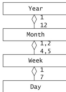
Figure 5-4 A naive model of the Gregorian calendar (UML class diagram).
