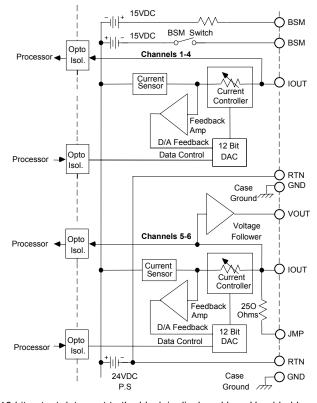
16-bit output data sent to the block is displayed by a Hand-held Monitor as an integer. The block's configured scaling determines the corresponding output signal value.
