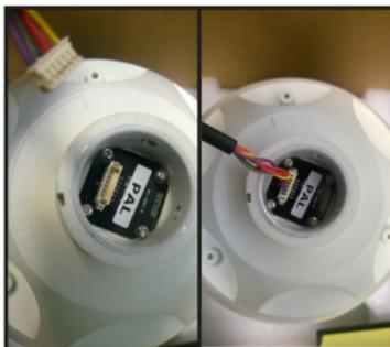
7. Re-attach the main camera to the bracket. To do this, use a cross head screw driver and turn screws in clockwise.
