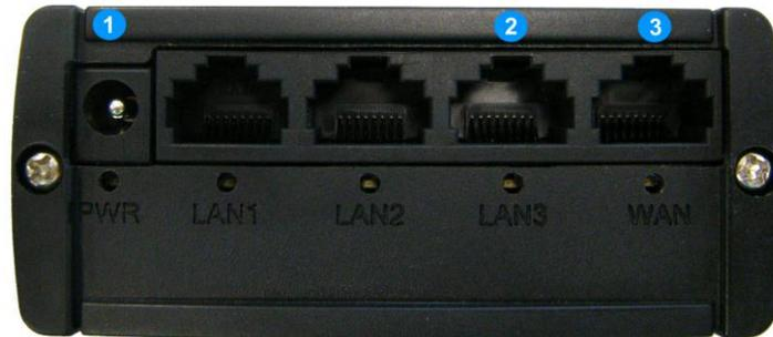
RUT5xx can be powered from power socket and over Ethernet simultaneously. Power socket has higher priority meaning that the device will draw power from power socket as long as it is available.
