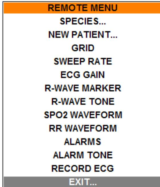
3. Use the UP/DOWN switches on the PC-Vet keypad to select the function and then the press the SELECT switch to choose the option. Repeat the process for each function. *NOTE: These functions may also be selected from the PC-Display toolbar or menus.*
