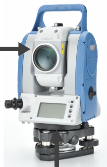
[1] Label for Laser pointer and Distance meter of Focus 8 2"
