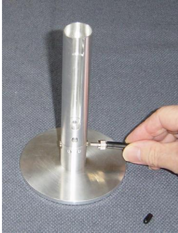
Figure 2. Connecting the cable to the pipette holder.
