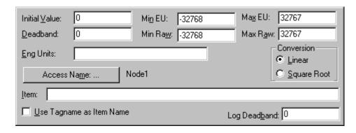
For integers fill in the Min EU, Max EU, Min Raw and Max Raw fields. These fields control the range of values that will be accepted from the Server and how the values are scaled. If no scaling is desired, Min EU should be equal to Min Raw and Max EU equal to Max Raw.
