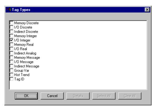
To access FESTOIPC device items, the type must be **I/O Discrete**, **I/O Integer** or **I/O Message**. Select the Tag type.
