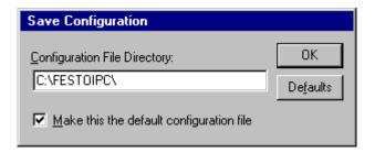
This dialogue box displays the path where the Server is going to save the current configuration file. The path may be changed if necessary. Also, the path can optionally be recorded in the **WIN.INI** file by selecting the **Make this the default configuration file** option. Doing so it will allow the FESTO IPC Server to find the configuration file automatically each time it is started.
