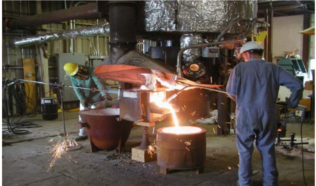
Figure 5-27: Manual Measurement of Temperature of Molten Iron
