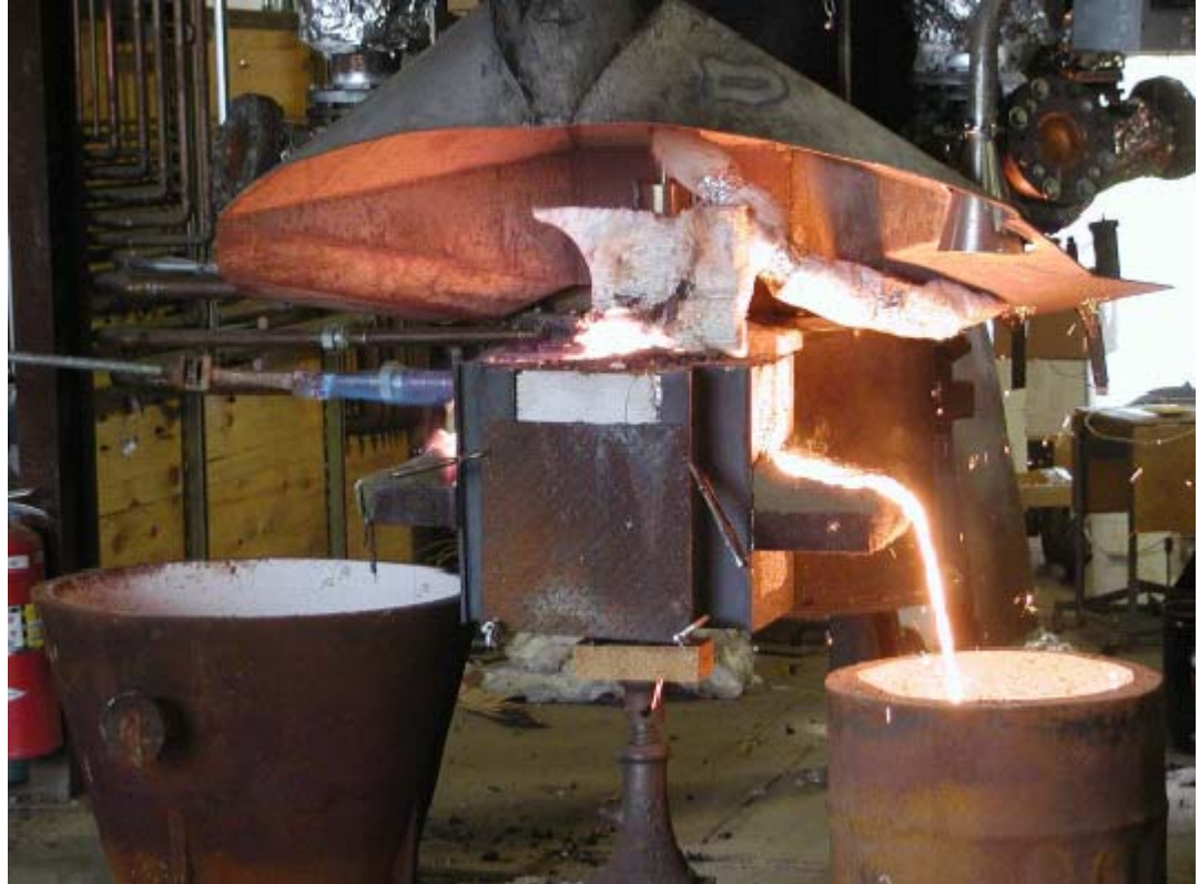
Figure 5-29: A Dip Thermocouple for Continuous Temperature Measurement
