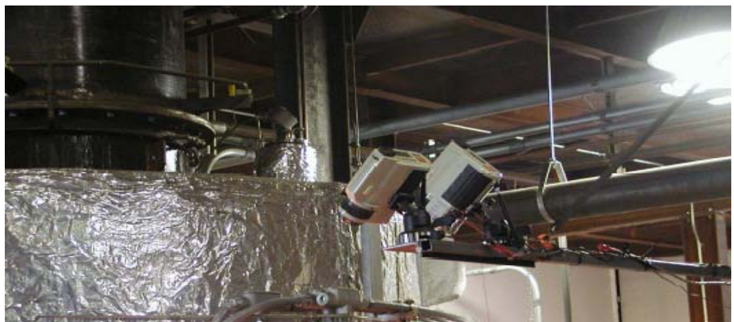
Figure 5-28: Optical Pyrometers for Continuous Measurements of Iron Temperature
