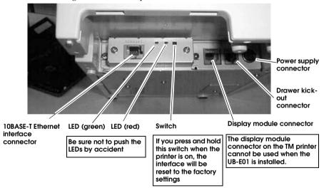
Note: This photograph shows the TM-H6000 printer with the UB-E01 installed.
