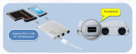
As the Picture shows, two external port is used, one is Expresscard, you can plug into two different sizes type of ExpressCard, 34/54, the other one is Thunderbolt interface, plug into the motherboards which include the Thunderbolt port.
