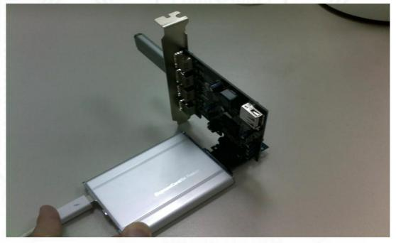
After plugging into thunderbolt port, you can check the PCI list and see the PCIe information as the Picture shows below, It means PCIe signal is recognized, then you can use some Peripheral PCIe equipment, for example, here is the PCIe to USB 4-ports module, then you can find USB Flash Disk on your desktop.
