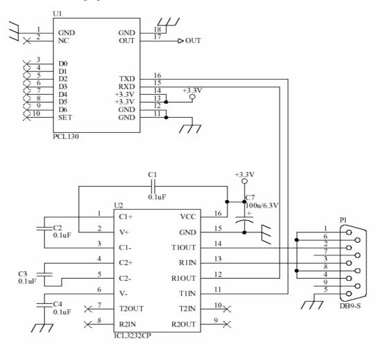
Note: The U2 level conversion IC is ICL3232CP manufactured by INTERSIL. The other ICL32XX series of level conversion ICs are also usable.
